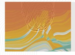
2D seismic snapshot and shot gather of the Marmausi2 model using SeisRTM isotropic modeling
