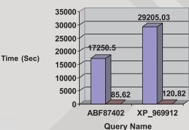
For two sample sequence searches against swissprot database, the RC based search was found to be around 200 times faster than a CPU-only solution.
