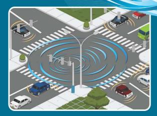
An indigenous Dedicated Short Range Communication (DSRC) System for vehicles comprising of On Board Unit and Road Side Unit with DSRC Software Stack. The system would enable two-way communication that can contribute to safer driving and also provide various applications that use the secure Vehicle to Vehicle (V2V) communications and Vehicle to roadside Infrastructure (V2I) communications.
