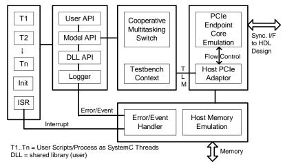
This eliminates the need for two back-to-back instances of PCIe Endpoint Cores and additional testbench creation in HDL. The improved overall simulation speed (by factor of ~10) and reduced memory usage (by factor of ~5.5) results are quite encouraging to apply same model to verify other designs having similar interconnect. The testbench complexity was transferred from HDL to external processes enabling efficient test-suite development for simulation.
