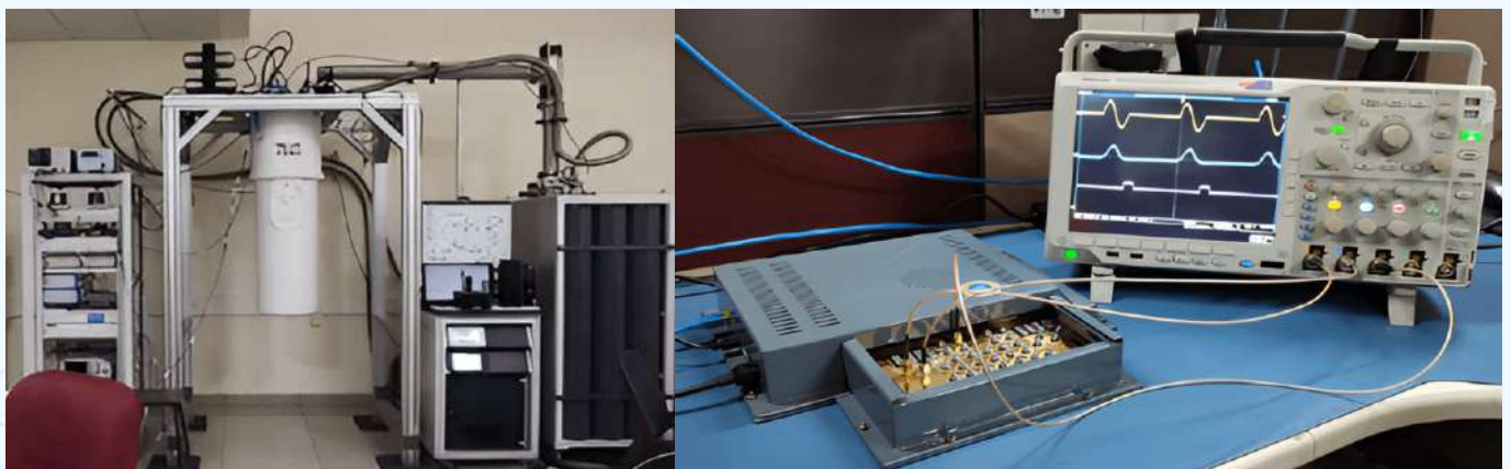
FPGA based control and measurement hardware for 4-qubit superconducting based quantum computer
