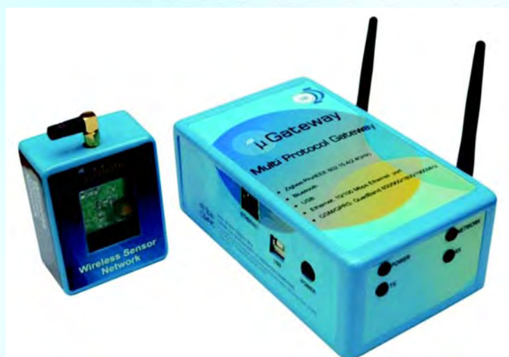
WSN with low power sensor mote and multi-protocol gateway
