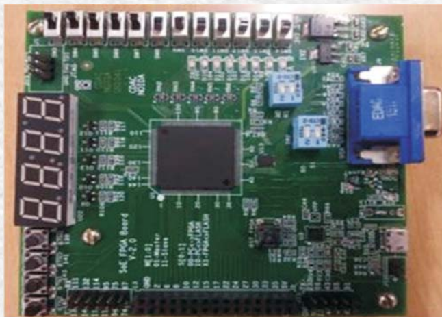
Low cost FPGA Development board featuring Xilinx Spartan-6 FPGA
