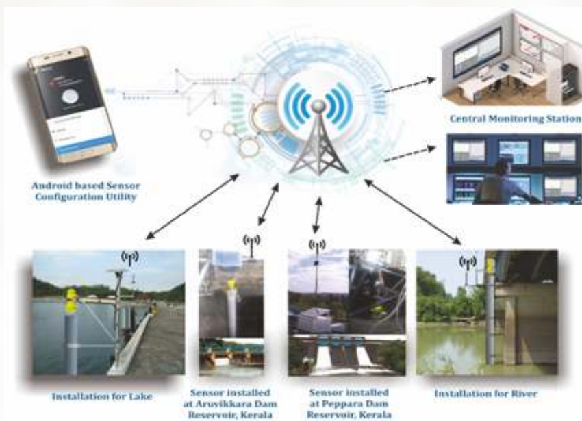
NIRCHHARI - Ultrasonic Level Sensor
