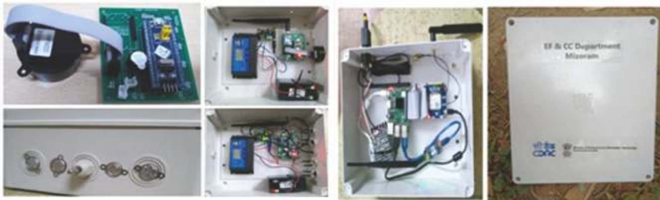
Forest Fire Wireless Sensor Node
