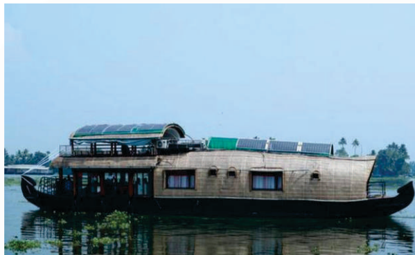
LVDC powered Houseboat (left), Flexible Solar Panels on rooftop (Right)
