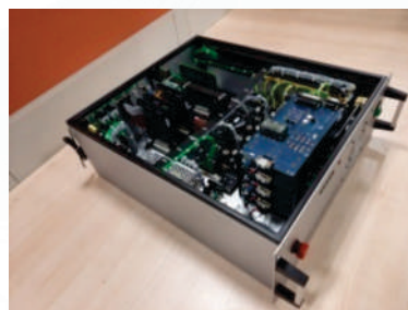
Automated Test Equipment for Magnetically Suspended Momentum Wheel Test Station (ATE-MSMW)
