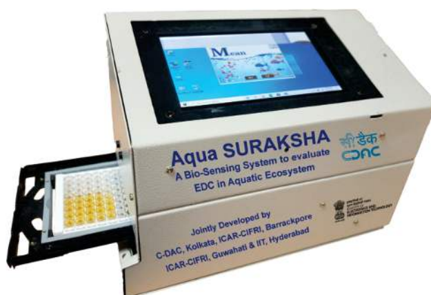
Aqua SURAKSHA - a Bio-Sensing system to evaluate Endocrine Disrupting Chemicals in Aquatic Ecosystem
