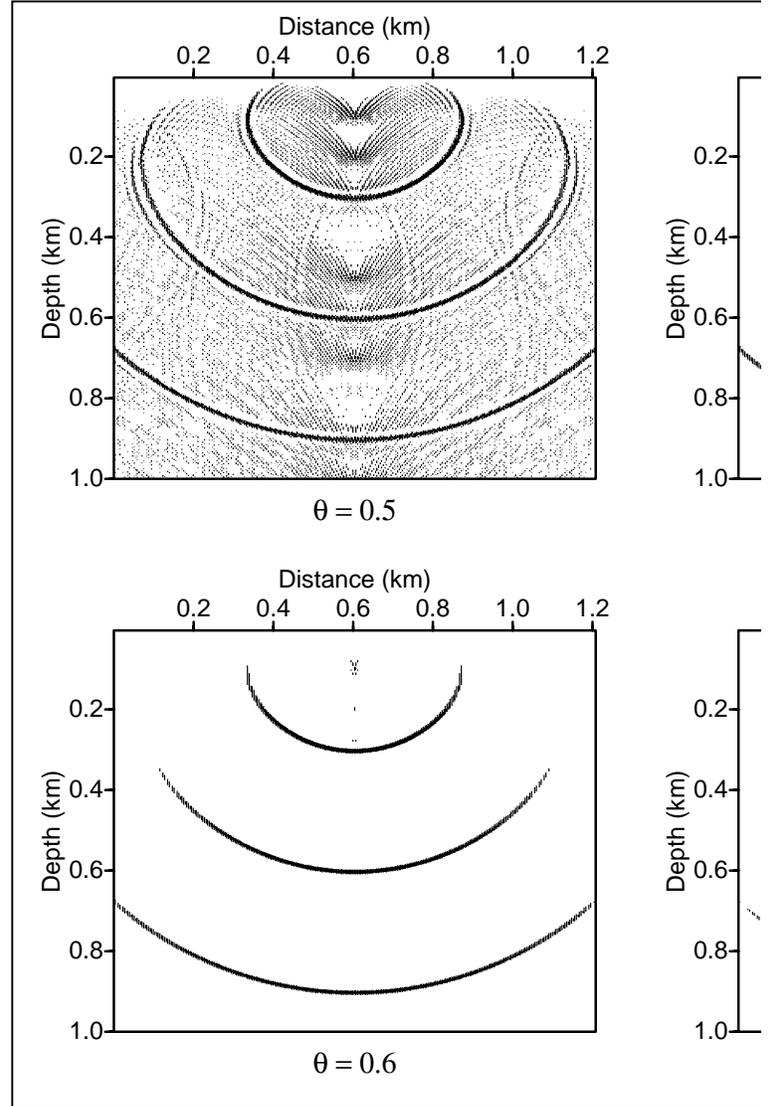
Figure 1: Impulse response of migration algorithm for different values of  $\theta$ . As the value of  $\theta$  increases, steep dips are also attenuated with the increase in  $\theta$  where
