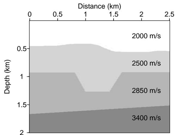
Figure 2: Velocity model used for the generation of synthetic data set.
