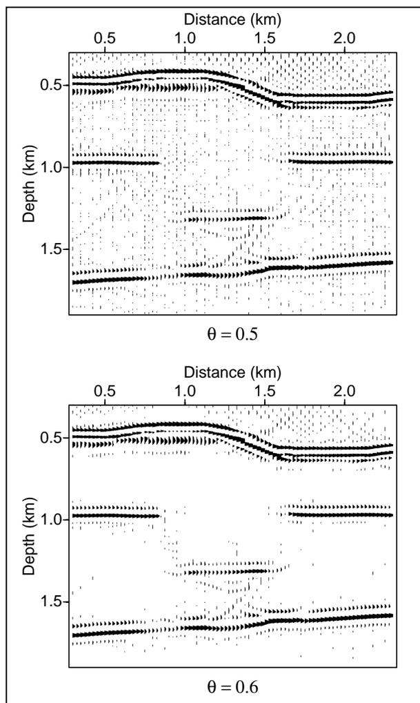
Figure 4: The migrated seismic sections of the stacked data shown in Figure 3 for  $\theta=0.5$  and  $\theta=0.6$ . Notice the reduction in evanescent energy for  $\theta=0.6$ .
