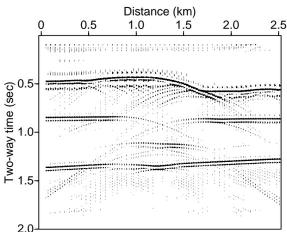
Figure 3: A CDP stacked section of the synthetic data set.
