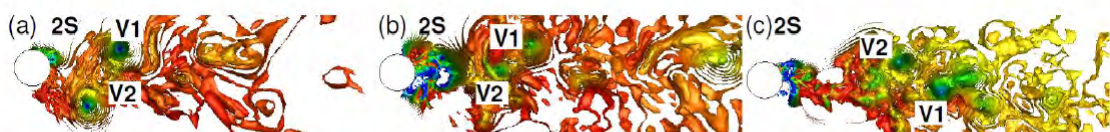
Figure 2. U^* = 5.0 , 3D –VIV of a cylinder: Instantaneous pressure iso-contours (a) Re = 5.0 \times 10^4 (b) Re = 1.5 \times 10^5 and (c) Re = 3.0 \times 10^5 at an instant when the displacement of the cylinder is at its maximum position.
