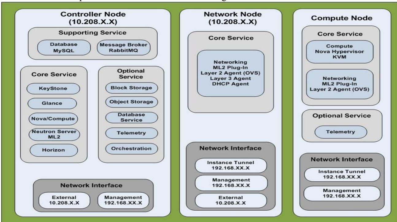
**Fig 2. Shown the Service running at the nodes**
