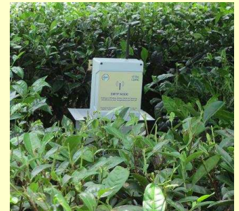
WSN Sensor Module at field
