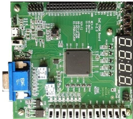
By default the board is powered from a +5V supply from USB cable. Built around a Xilinx Spartan-6 FPGA the board provides, a complete ready-to-use hardware suitable for hosting circuits ranging from basic logic devices to complex controllers. A large collection of on-board I/O devices/interfaces and all required FPGA support circuits are included, so countless designs can be created without the need of any other components. The design can be controlled and
