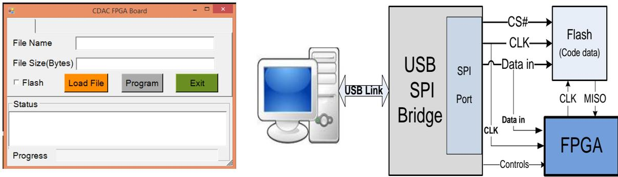
After power-on, the FPGA on the development board must be configured before it can perform any useful functions. During configuration, a “bit” file is transferred into memory cells within the FPGA to define the logical functions and circuit interconnects. The free ISE/WebPack CAD software from Xilinx can be used to create bit files from VHDL, Verilog, or schematic-based source files.
