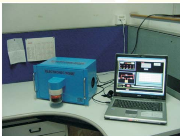
E-Nose with illumination based heating
